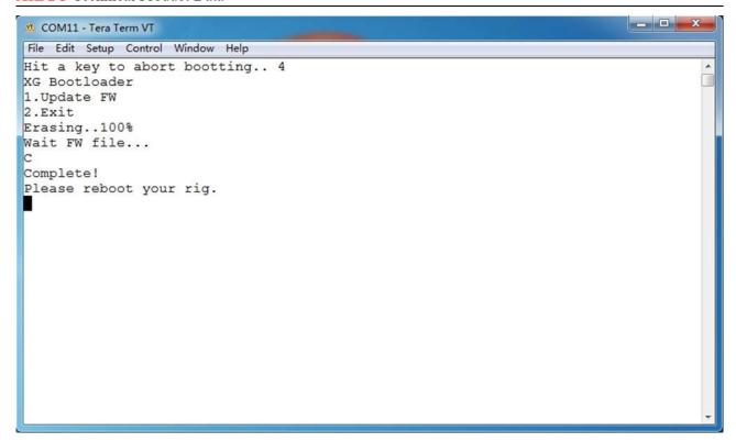
Fig. 11 Information displayed in the software window after the firmware is sent
