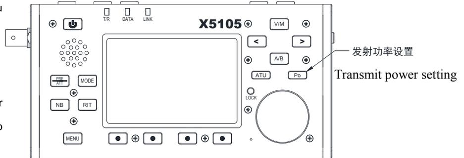
◆ When using the X5105 transceiver for the first time without knowing the current antenna state, please reduce the set transmit power value as far as possible.
