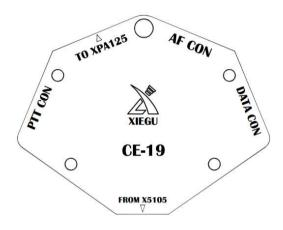
PTT CON PTT signal / BAND signal output. This interface PTT signal is completely isolated from the host, providing a "low level" trigger
