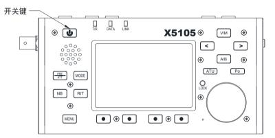
♦ Hard reset: when the host system is in a dead state, such as button not responding, or unable to exit the launch state and button not responding, Long press switch button and hold for more than 8 seconds, reset MCU and force shutdown.
