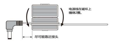
Note: 电源线在磁环上绕两圈(Wrap around two turns.);尽可能靠近接头(As close as possible.)
